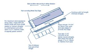
Trim shingle at alignment slit 12" (305mm). Position shingle on top of cut-out of underlying shingle so that there will be 7 1/2" (191mm) of each shingle exposed. Factory applied self-sealing dots on lower courses are designed to seal down the shingle tab in an upper course. NOTE: Shingles may be laid from either left or right hand side. Start at either rake edge with shingles having 12" (305mm) trimmed from rake.
