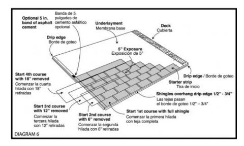
Fourth Course: Cut 18" off a shingle and apply the right half over the third course, flush with the left rake edge, exposing 5". Proceed with full shingles across the roof, maintaining 5" exposure on the course below.
