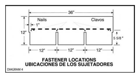
Re-Roofing Application (second shingle layer): Requires the same nail placement as New Roofing but NAILS MUST BE A MINIMUM OF 1-1/2" LONG. NAIL PLACEMENT IS IMPORTANT FOR WIND RESISTANCE. INCORRECTLY PLACED NAILS MAY VOID WIND COVERAGE OF WARRANTY.
