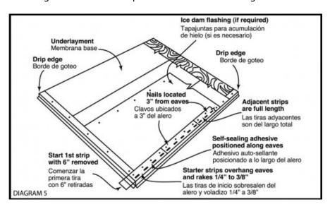
First Course: Begin first full shingle at lower left rake of roof or right of vertical chalk line and continue course across roof with full shingles laid flush with starter course and fastened with 4 nails placed as specified. Note: An optional band of asphalt plastic cement meeting ASTM D-4586 may be applied to the rake of the roof with each shingle course to enhance wind resistance and to resist wind driven rain. See Diagram #6.
